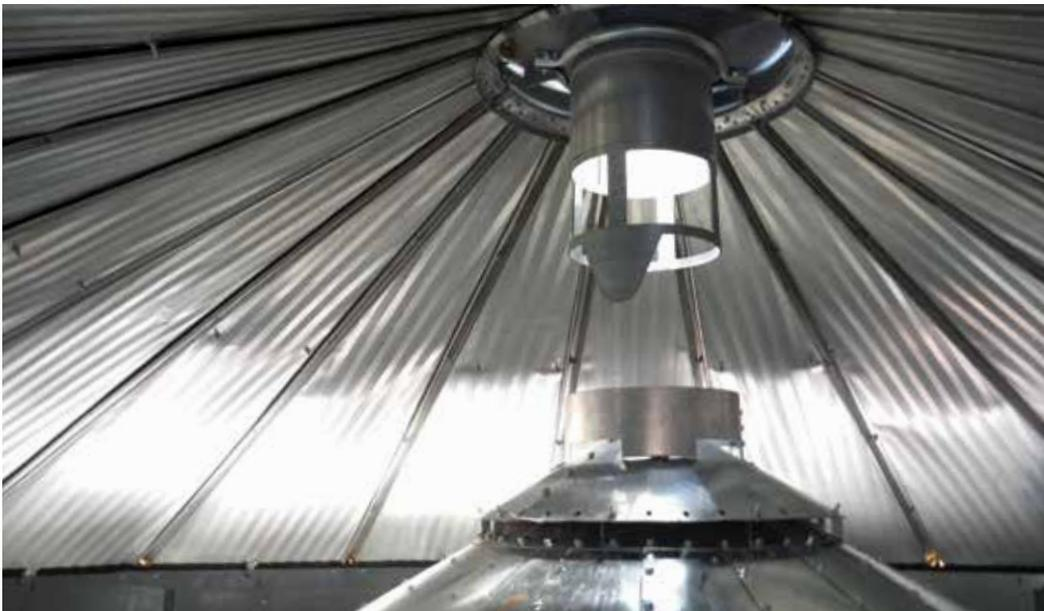
Grain moves down out of the garner area, and enters 12-3/4 inch wide grain drying columns in the heat section of the dryer.
