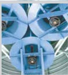
Internal inline, mixed flow centrifugal blowers deliver high volumetric airflow to the pressure heat and vacuum cool sections. **SEE PAGE 10 FOR MORE INFO.**
